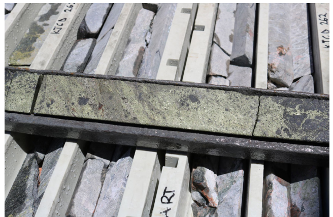
Figure 3. Chalcopyrite and pyrite mineralisation from KJCD273 at ~586 m depth (assayed at 11% Cu).
