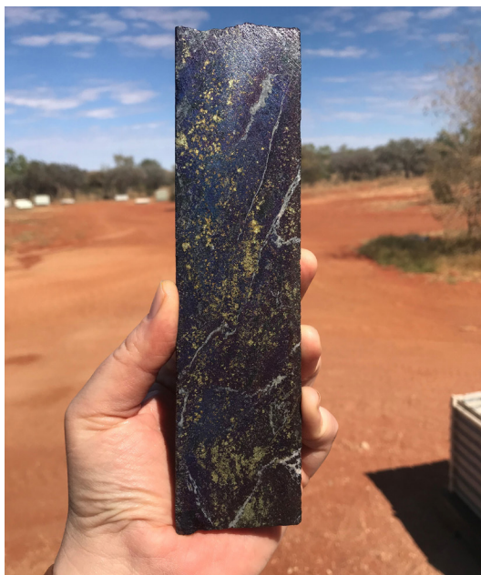
Figure 2. Bornite and chalcopyrite mineralisation from KJCD358 at ~358 m depth (assayed at 34% Cu).
